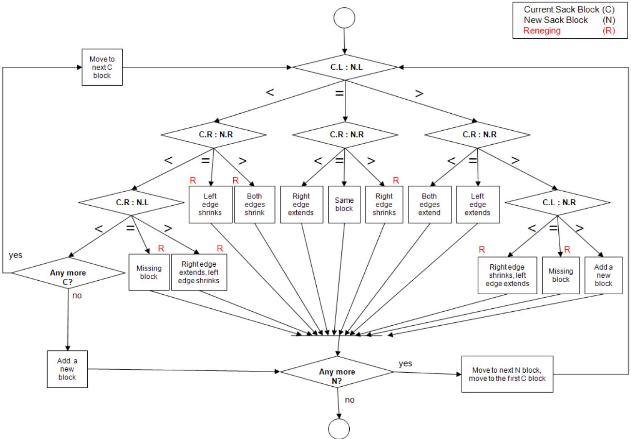
**Figure 3. Data Reneging Detection Model**
