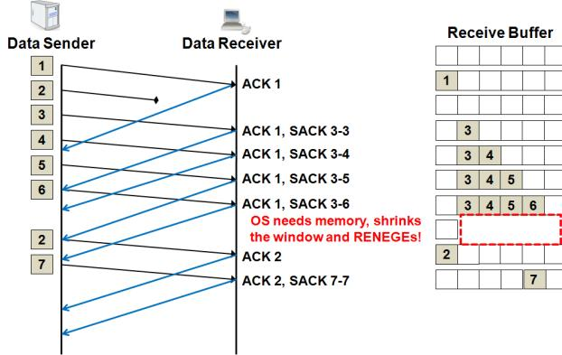
**Figure 1. Detecting data renegeing at SCTP data sender**
