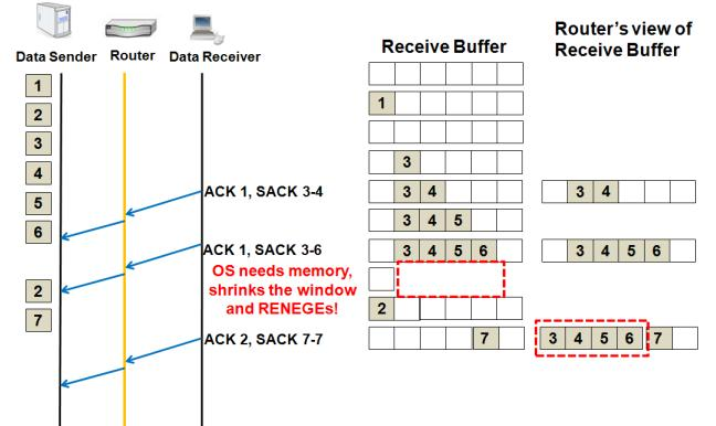
**Figure 2. Detecting data renegeing by an intermediate router**
