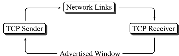
Fig. 1. Established and widely accepted TCP control loop model. Its limitation is that it does not adequately take the sender and receiver operating systems into consideration. In this work, we concentrate our efforts on monitoring the receiver and the effects its operating system can play.
