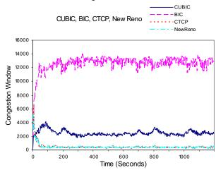
Fig. 2. Congestion window curves for CUBIC, BIC, CTCP and NewReno flows. A congestion window curve represents the sum of 20 flows of a type
