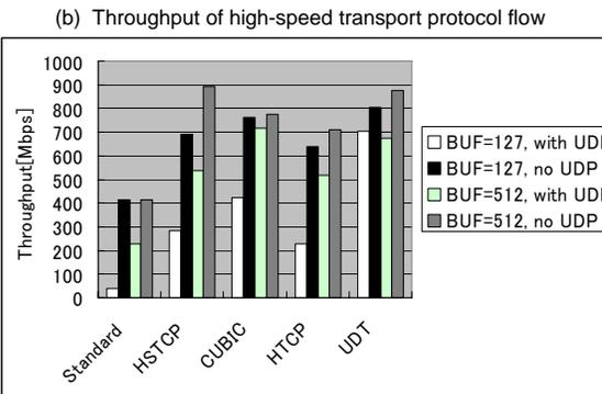
Fig. 13. Jitter of UDP flow and throughput of high-speed transport protocol flow in case 1
