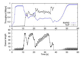
Figure 5: Throughput of RAPID and TCP cross traffic starting at 10 seconds.
