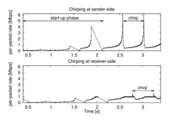
Figure 4: Per-packet rate of one continuous RAPID transfer with 32 pkt/chirp over an 1 Mbit/s link.
