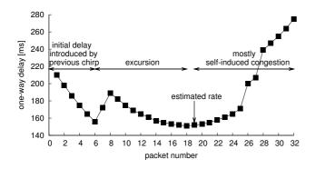
Figure 2: Queuing delay of a 32 packet chirp with TCP cross traffic.
