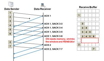
Figure 1. Detecting data reneging at SCTP data sender
