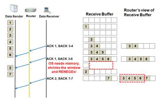
Figure 2. Detecting data reneging by an intermediate router
