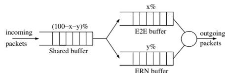
Figure 3: Egress buffer scheme for IP-ERN routers
